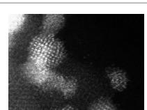
The shape of gold: The title catalyst has been prepared through a colloidal deposition method. Scanning transmission electron microscopy studies confirmed that for the catalyst, gold clusters with a bilayer structure and a diameter of about 0.5 nm are not mandatory to achieve the high activity (see image).
