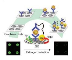
Don't FRET when I GO: Sensitive and selective rotavirus detection is achieved by using the photoluminescence of a graphene oxide (GO) array. The target cell was captured by the rotavirus-specific antibody immobilized on the GO array, and the binding event was monitored by observing the fluorescence quenching that results from fluorescence resonance energy transfer (FRET) between GO and gold nanoparticles linked to the antibodies (see picture).
