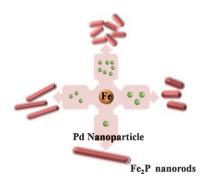
Playing a dual role as a catalyst that destabilizes Fe nanoparticles to form soluble precursors in situ and as a catalytic center for nanorod growth allows Pd nanoparticles to transform Fe nanoparticles and a P source into Fe<sub>2</sub>P nanorods (see scheme). The diameter and length of the Fe<sub>2</sub>P nanorods can be finetuned by means of the diameter of the Pd nanoparticles and the Fe/Pd ratio, respectively.
