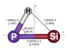
Curiouser and curiouser: By combining high-resolution molecular spectroscopy in the centimeter and millimeter wave regions, and high-level coupled-cluster quantum-chemical calculations, the structure of the HPSi molecule has been determined. The bridged geometry of HPSi is in remarkable contrast to that of the C and/or N analogues, such as HCN/ HNC, HCP, and HNSi, which are all linear.
