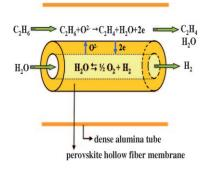
Burns at both ends: By coupling water splitting and ethane dehydrogenation in a perovskite (BCFZ; BaCo<sub>x</sub>Fe<sub>y</sub>Zr<sub>1-x-y</sub>O<sub>3- $\delta$ )</sub> oxygen-permeable membrane reactor, hydrogen from water splitting was obtained on one side of the membrane, and ethylene was produced simultaneously on the other.
