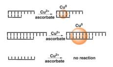
A helping strand: A method to selectively form copper nanoparticles in solution using double-stranded DNA has been developed. The size of the nanoparticles is controlled by the length of the dsDNA template, and single-stranded DNA did not act as a template (see scheme). Single-stranded overhangs in dsDNA were used to prepare a nanostructure in which two metallized dsDNA segments were linked together by a nonmetallized rigid
